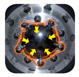
Stretch the squirrel in direction of arrows. Start fitting the squirrel from the least accessible position (ie from the bottom of a wheel). Weave the squirrel alternately inside every other wheel-nut working upward towards the top of the wheel.
