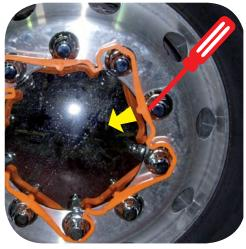
Using a screwdriver, lever the last part of the squirrel into position while pushing firmly towards the rim.
